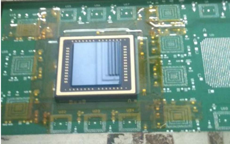
Figure 34. Ceramic land grid array (LGA) package with SnPb solder bumps assembled onto PCB.
