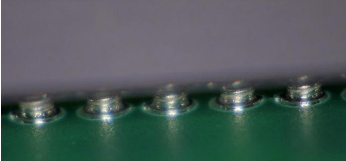
Figure 29. Representative photomicrographs of solder joint quality after assembly for microspring coil column CGA1571.
